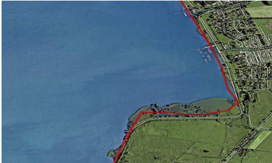
Figure 1: Using aerial imagery from Google Maps the OpenStreetMap representation of the Dummer See in Lower Saxony, Germany is overlaid
