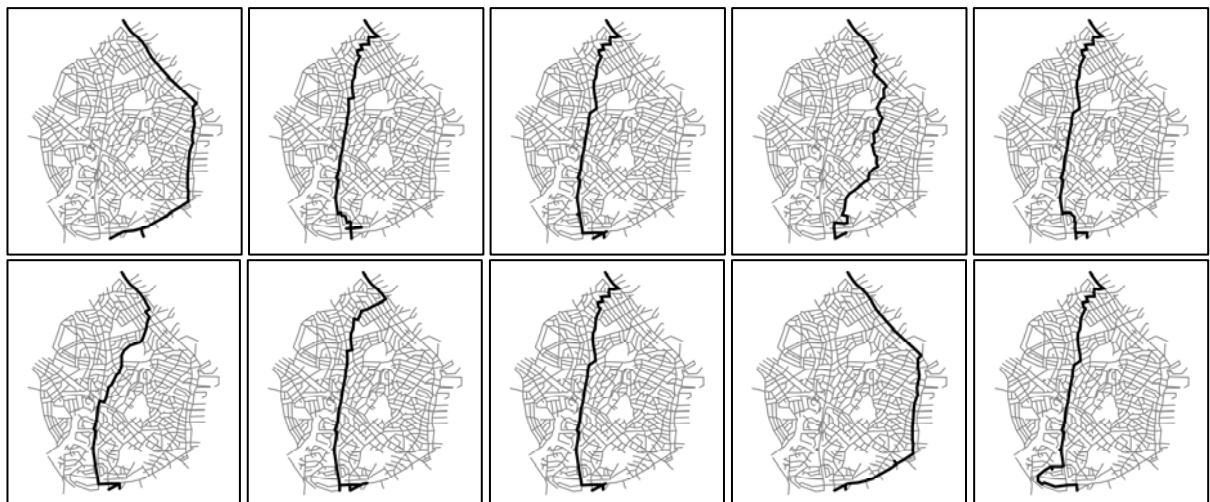
Figure 5. Paths realized according to the arc-admissibility rule expressed by Equation 2. Note that some nodes and arcs may be visited more than once in each path.
